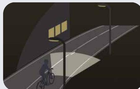
Standard beam (low-beam) is ideal for riding in the **city**, while preventing incoming users with excessive glare.
