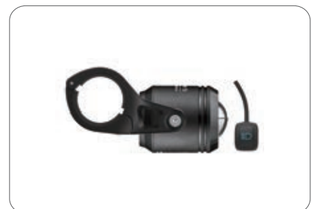
Light model: HEAE200R Holder: Side Cable Length: 1400mm Control Switch : 300mm+ Switch bracket /mount: Ø22.2mm Mount: Handlebar mount (PHB31850) Mount size: Ø31.8 & 35mm Waterproof connector (ct22) SKU No. AE2003
